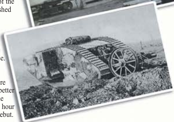
Above from top to bottom: this C Battalion Female Mk I came to grief when it lost a track during the Battle of Flers; a new Mk I boarding a train at Fosters factory, the Russian script on the side is supposed to fool the Germans into thinking that they were water carriers destined for Russia; a damaged Mk I after Flers, note the missing rear wheel from the steering gear.
