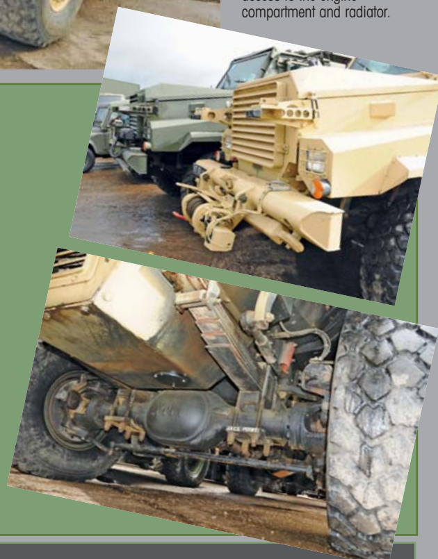
Below: looking at the front of two of the Tempest MPVs at Withams, we can see the front mounted winch in the raised (far vehicle) and lowered (nearest the camera) positions, which provides access to the engine compartment and radiator.
