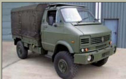
Reynolds Boughton RB 44 Truck Cab Pickup R.H.D, Permanent 4x4, 5 speed g/box, hi/lo box differential Lock, power steering, carries 2250 kgs, Perkins Phaser 110T T/Diesel engine, Mileage from 37,000, Guide price from £3,750 (100 Available)
